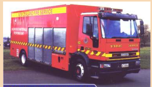
IVECO - Hazardous Materials Response Unit Is specially designed to carry equipment for use at emergencies involving dangerous chemicals. It also carries special gear to help firefighters rescue people. • Model: ML150E335 • Engine: IVECO 8060.455 • Year: 2001
