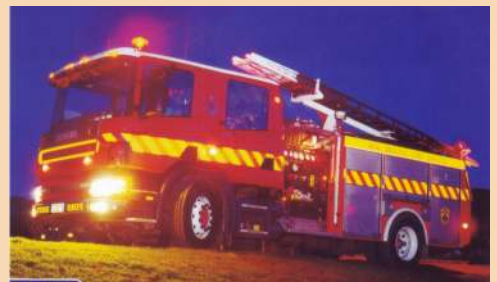
SCANIA • REG No: XD3574 • Year: 1998 • Pump Output: 75 litres per second • Water Tank Capacity: 1,350 litres • Engine Power Output: 191kw @ 2000rpm • Weight: 13,900kg
