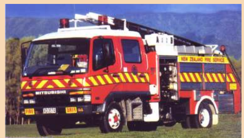
MITSUBISHI • REG No: XD3574 • Year: 1998 • Pump Output: 37 litres per second • Compressed Air Foam • Water Tank Capacity: 2,000 litres • Engine Power Output: 140kw @ 2900rpm • Weight: 9,900kg
